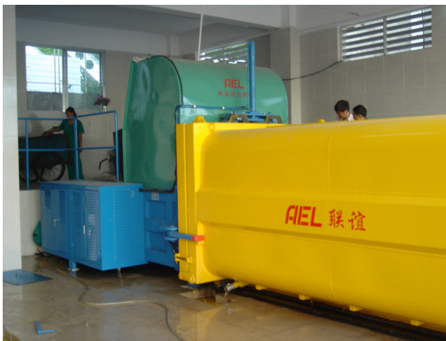
Refuse compaction system Infeed option: Rear platform 垃圾压缩系统后平台上料模式
