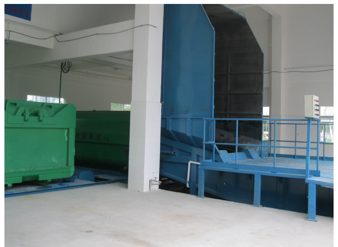
Model 3200: Refuse compaction system Infeed option: Front platform 3200 型前平台上料压缩系统
